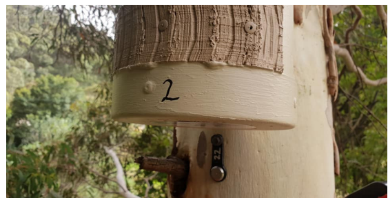
External hygrochron installed below hollow
