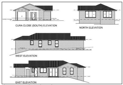
Figure 8: Unit 3 Elevations
