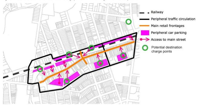
Figure 4 Locations suitable for destination charge points within the Lithgow Main Street precinct
