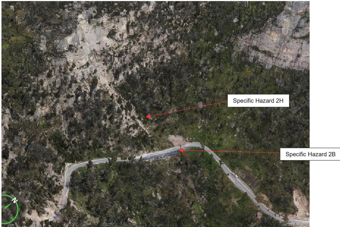
Figure 1: Aerial photogrammetric view of Hazard 2B below Hazard 2H from 15.11.2022 Aerial Survey
