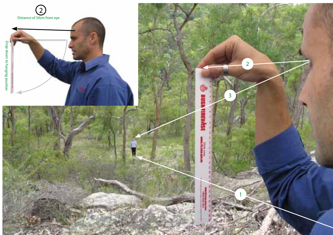
Fig 4. Simple slope assessment methodology.
