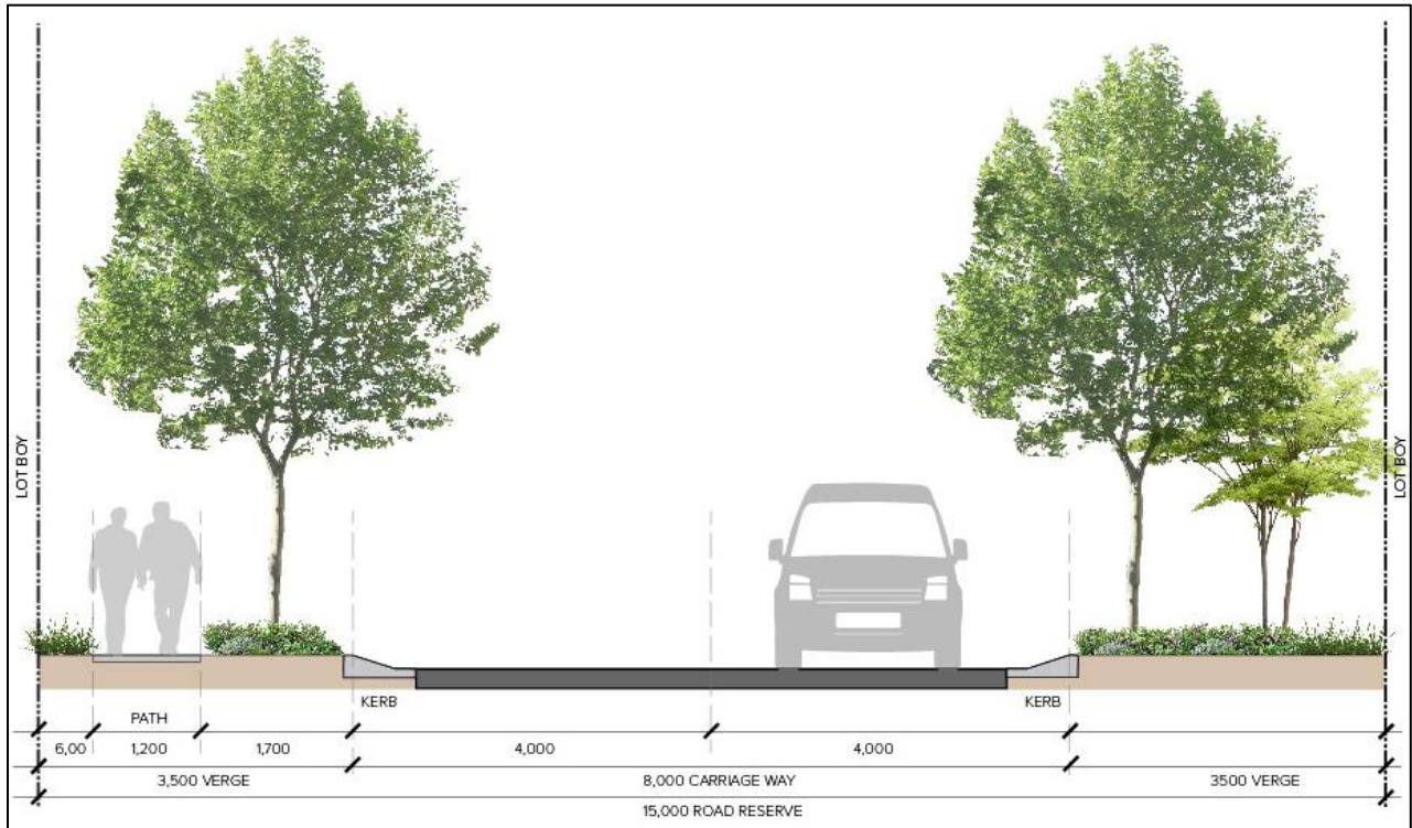
Figure 24. Road Type 1 - Cross Section
