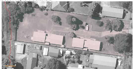
The flood level for this area is 928AHD and adding a 0.5m freeboard the required flood planning area is shown in red. No structure will be erected within this area and the finished floor levels for Units 16, 17 and 18 are above 931AHD. Open pool type fencing is also proposed which will minimise impact of flood waters. The proposed development will not impact on the flood waters subject to the condition of consent:
