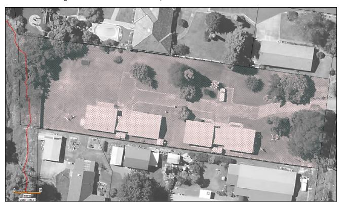
The flood level for this site is 928AHD and adding a 0.5m freeboard the required flood planning area is shown in red. No structure will be erected within this area
