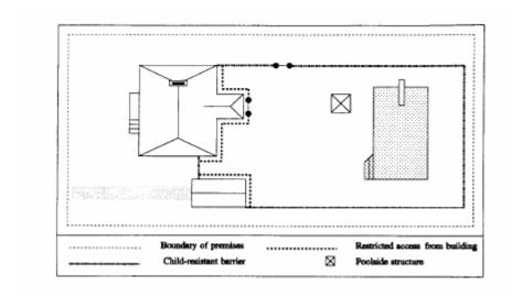
Figure 6: Existing Swimming pools and new swimming pools on very small properties (i.e properties with a site area less than 230 square metres)
