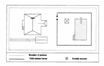
Figure 4: Boundary fencing used together with a fence to isolate the pool from the dwelling.
