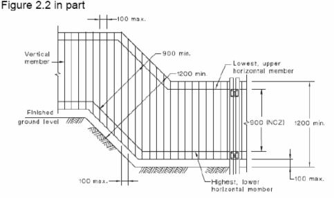
NOTE: On sloping sites, the fence height is to be measured perpendicular to the ground line.
