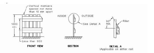
FIGURE 2.4 FENCE WITH HORIZONTAL MEMBERS PROJECTIONS OR INDENTATIONS NOT ACTING AS A HOLD FOR CLIMBING
