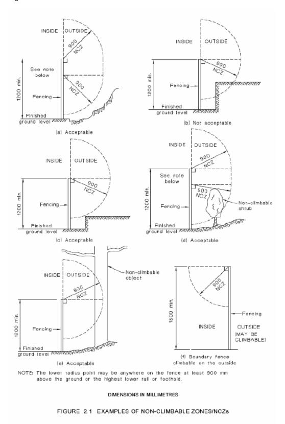
Fences using perforated materials or mesh, with apertures not greater than 13mm shall have an effective height not less than 1200mm. Fences using perforated materials or mesh with apertures greater than 13mm but not greater than 100mm shall have an effective height not less than
