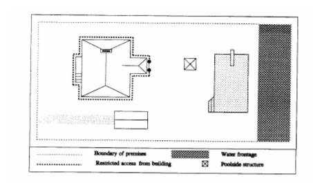
Figures 7 and 8 show all of the windows and doors in the dwelling being made to comply with Clauses 2.7 and 2.8 of AS 1926.1 – 2007 respectively.
