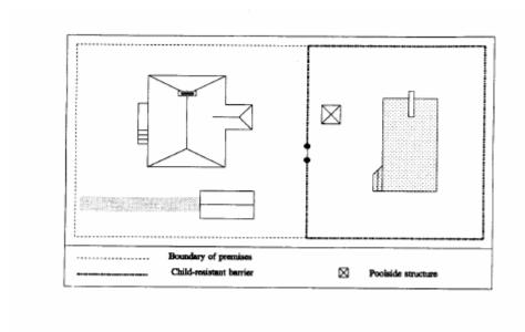
Figure 5: Existing swimming pools and new swimming pools on very small properties (i.e properties with a site area less than 230 square metres).
