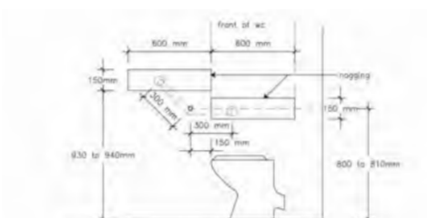
Figure 6(a) Toilet - Location of reinforcement
