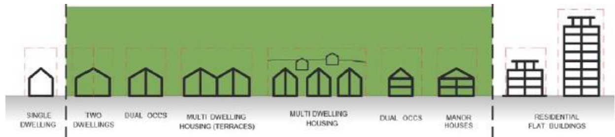
Range of residential types the Design Guide for DAs applies to (Guide Figure 1-1).
