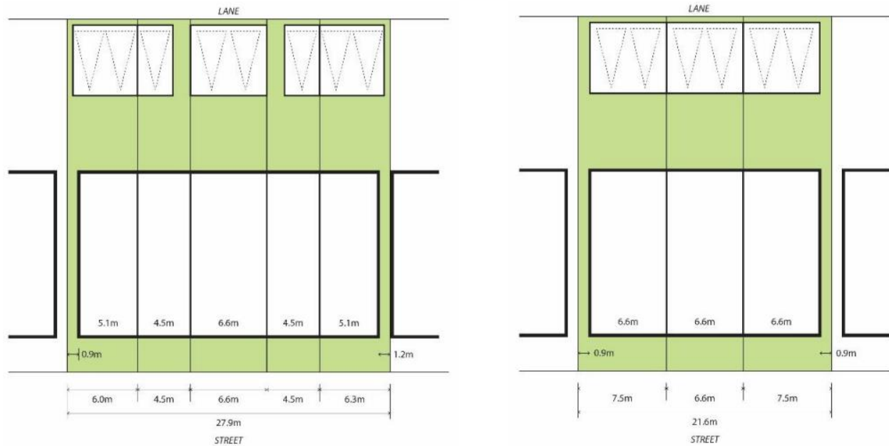
Figure 21. Two examples of lot subdivision for ‘sets’ of attached or abutting dwellings
