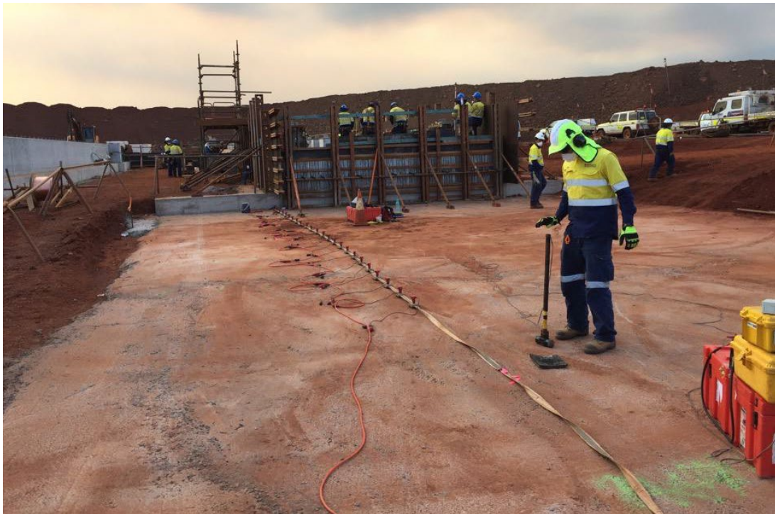
Figure 2: Collection of MASW Data Using a Land Streamer with 24 Geophones
