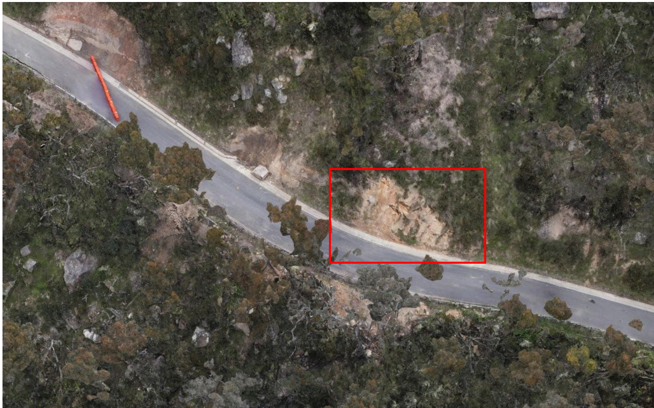
Event 81 - Aerial photogrammetry showing landslide, captured 15/11/2022.
