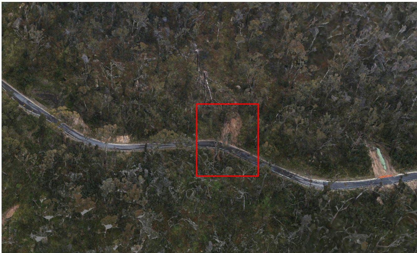
Event 70 - Aerial photogrammetry showing embankment failure, captured 13/12/2021.
