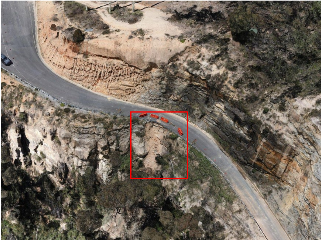
Event 68 - Aerial Photogrammetry showing embankment failure, captured 13/12/2021.
