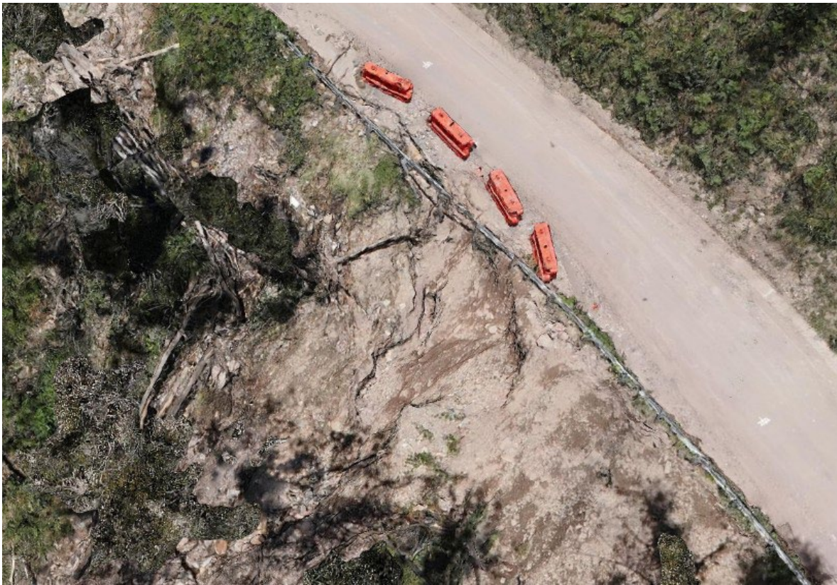
Event 70 - Aerial photogrammetry showing embankment failure, captured 13/12/2021.
