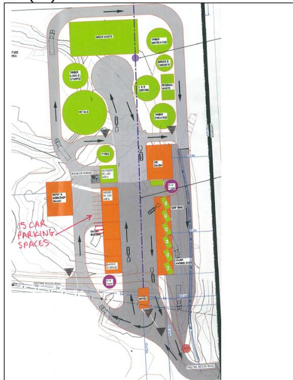
**Figure 8 – Car and Truck Parking Configuration**
