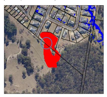
The detention basin on Council's land is designed to capture stormwater in a 1 in 100 year event, while overland flow towards the detention basin on the applicant's land
