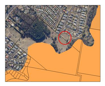
The area of the proposed earthworks is not within the mapped areas, which are all upslope from the area of the proposed works. Therefore there is unlikely to be any adverse impact on sensitive lands as a result of the proposed works.
