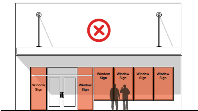
signage exceeds 30% (or 6m 2 ) or window surface area
