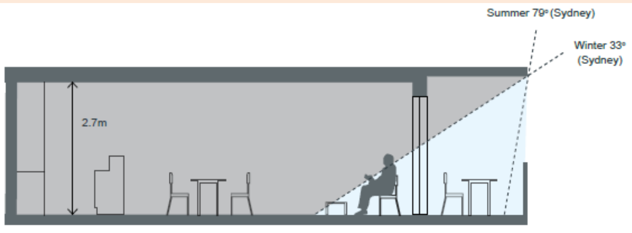
Example of how shading can affect winter & summer sun (SEPP65/ADG).
