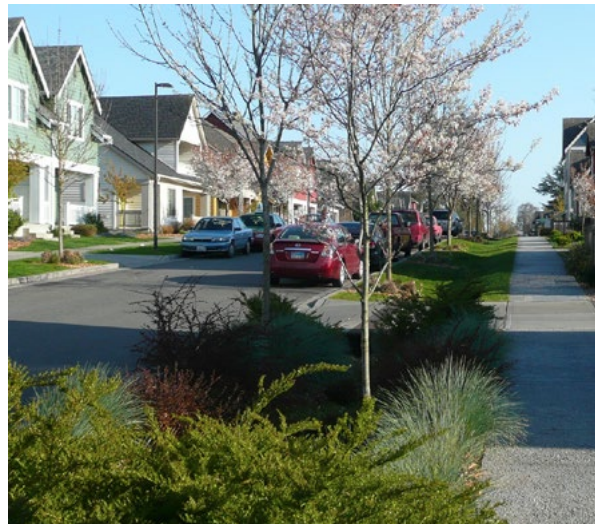
Figure 3-138 Swales can be attractive, and are able to filter and collect the stormwater
