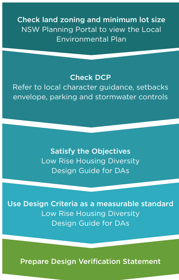
Figure 2-28 Workflows: Preparing a DA
