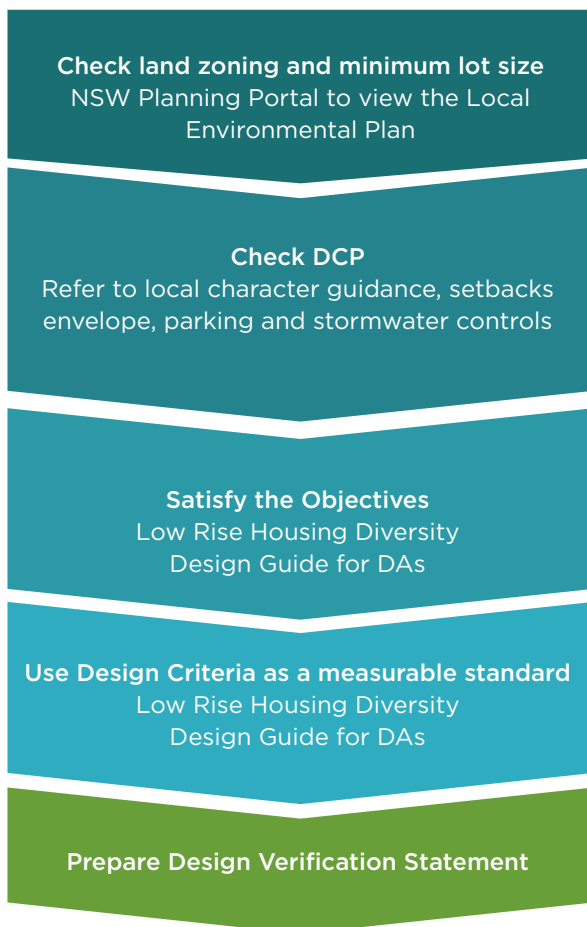
Figure 2-35 Workflows: Preparing a DA
