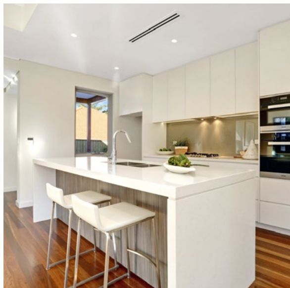
Figure 3-147 Clear space between bench tops makes it easier to use the kitchen
