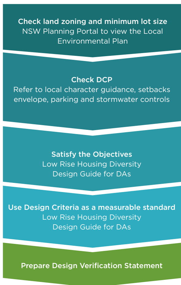
Figure 2-31 Workflows: Preparing a DA
