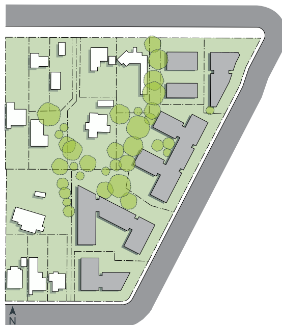
Figure 3B.1 Proposed buildings are sited to clearly address the street while maximising solar access to apartments
