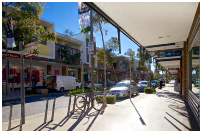
Figure 4T.1 Continuous awnings should be provided where there is high pedestrian activity e.g. in centres and along active frontages
