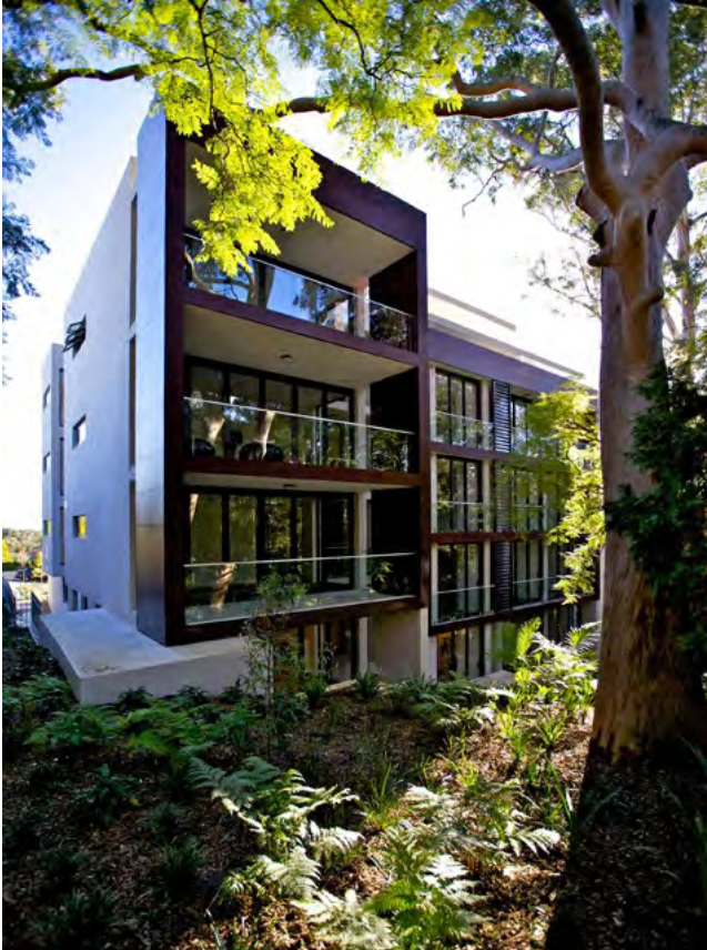
Figure 3E.3 Deep soil zones promote the growth of larger trees which improve amenity and local microclimate
