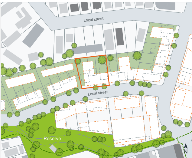
Figure 1B.6 The streetscape scale helps understand the impact of proposed development on streetscape quality and should show heights, setbacks, driveways and existing street trees. All proposals should address this scale
