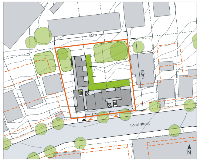
Figure 1B.7 The site scale is a detailed analysis of the development's immediate context and should include the site itself, the street it addresses and surrounding properties. All proposals should address this scale
