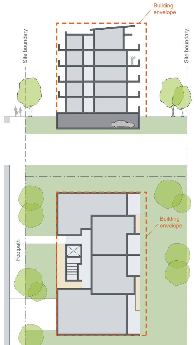
Figure 2B.2 Building envelopes define the 'container' within which a building is designed. They are a useful tool to gain an understanding of the future urban form and scale of an area. The gross floor area of the building is typically 25-30% less than that of the envelope
